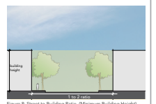
Figure 8: Street to Building Ratio (Minimum Building Height)
